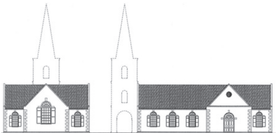
Exterior plan, with large east end window and conjectural bell tower, east and south elevations, 1733–62 (Courtesy of Richard Marks Restorations and St. Andrew's Parish Church. Drawn by Larry S. Leake, Richard Marks Restorations)
